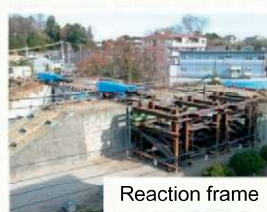
Figure 23.18 A full-scale model of GRS integral bridge constructed at Railway Technical Research Institute: (a) overall structure, (b) left-side abutment under construction, and (c) full-scale loading test performed in January 2012.
